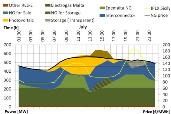
**Figure 13:** July day 2030 scenario for a setup that includes a pumped hydro storage facility. See main text for assumptions.
