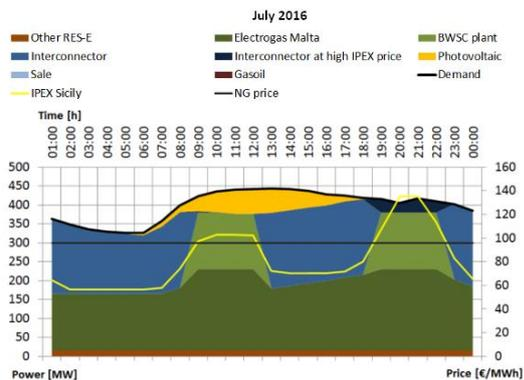
**Figure 5:** 2016 scenario for a day in July, with modelled IPEX curve based on a TERNA-based projection. See main text for assumptions.
