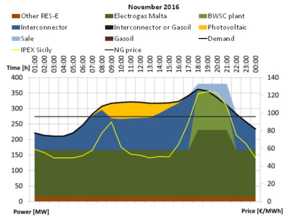
**Figure 7:** 2016 scenario for a day in November, with modelled IPEX curve based on a TERNA-based projection. See main text for assumptions.
