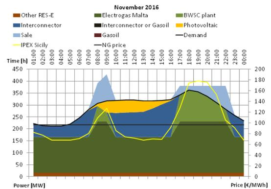
**Figure 8:** 2016 scenario for a day in November, with modelled IPEX curve based on a three percent annual growth projection. See main text for assumptions.
