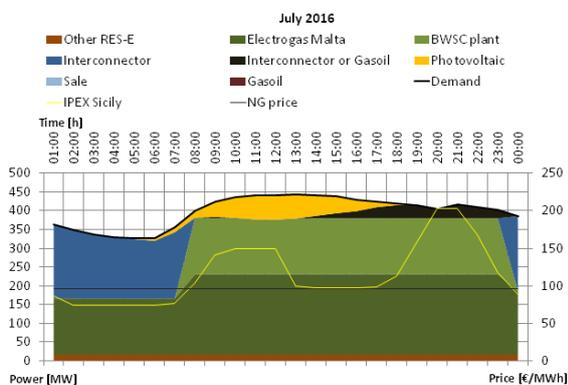
**Figure 6:** 2016 scenario for a day in July, with modelled IPEX curve based on a three percent annual growth projection. See main text for assumptions.
