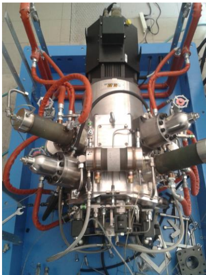
Figure 9: Photo of the High Energy Density Stirling engine proposed by FBK
