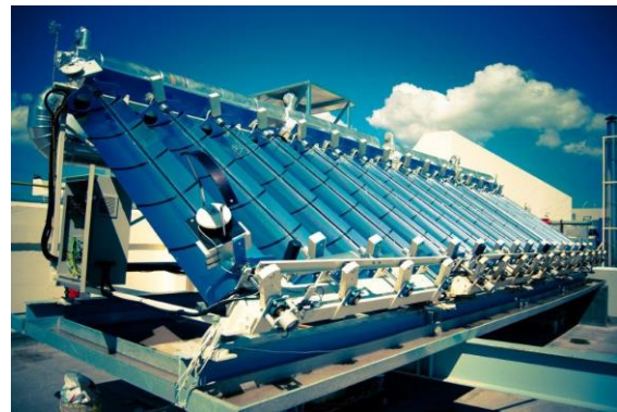
Figure 7: the DiGeSPo solar system
