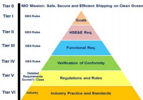
Fig. 3. Suggestions of modifying the IMO’s original concept for goal-based standards with six tiers [1].
