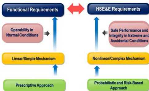
Fig. 2. Paradigm shift in design and engineering of ships and offshore structures [1].
