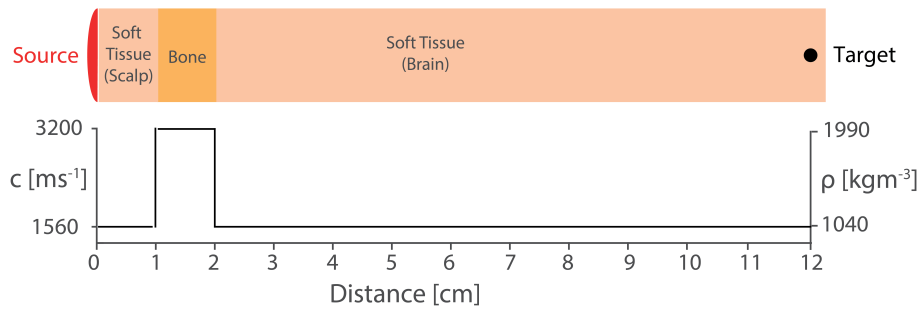
Figure 2.2: A scaled schematic of the simulation model used to evaluate the impact of numerical errors.
