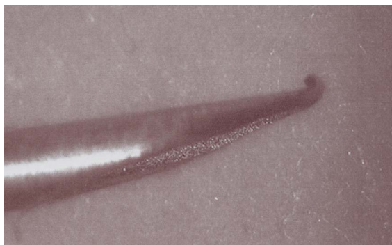
Fig. 2. XL Monoprotect® needle with non-preserved bevel after truncal block of the inferior alveolar nerve (40X).
