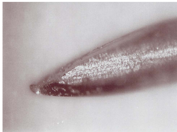
Fig. 1. Monoprotect® needle with non-preserved bevel after truncal block of the inferior alveolar nerve (100X).
