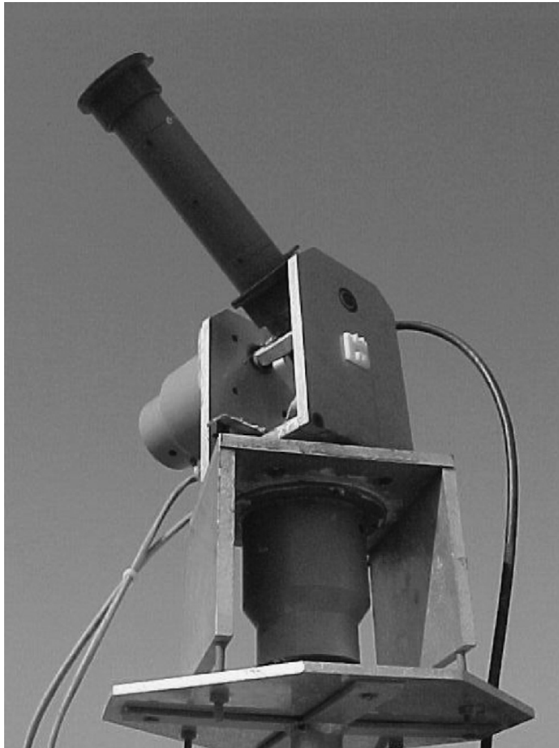
Fig. 2. The sun tracker mounted on the metal platform. The pass motors, radiance limiting tube and fibre optic can be seen.
