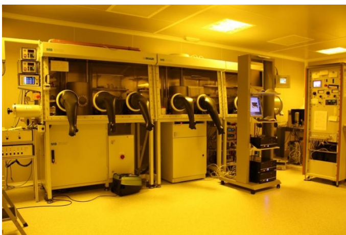
Fig 2.1 Nitrogen-filled glove box installed inside the clean-room at the Instituto de Ciencia Molecular (ICMol) of the Universidad de Valencia where all the devices were prepared and characterized.
