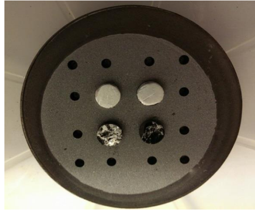
Figure 6.4: Powder pressed custom drilled target with doping pegs.
