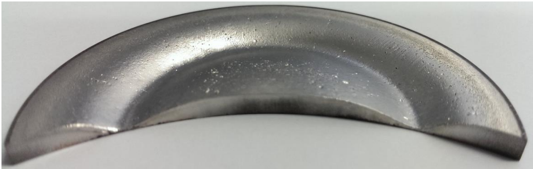
Figure 6.2: Unevenly eroded Ta magnetron target.
