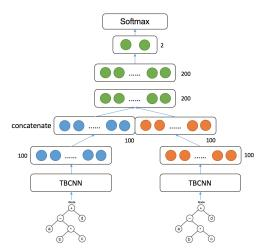
Figure 3: BiTBCNN architecture for program classification
