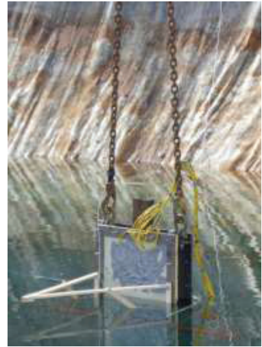
Fig. 1. (a) diagram of panel setup for underwater blast test; (b) photograph of panel being lowered into the water from crane without charge on pine frame.
