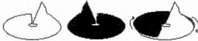
Maxwell's spinning disc set-up. Two different coloured pieces of paper, with slits on a radius, were slotted together. The final, spun colour was identified by the precise proportions from the two original colours.
