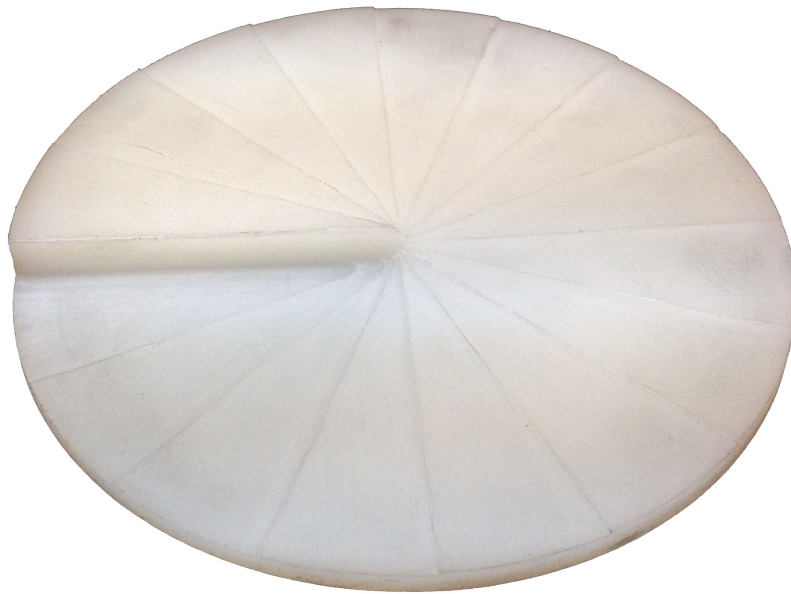
Figure 4.1: A polypropylene \Delta l = \pm 1 SPP.
