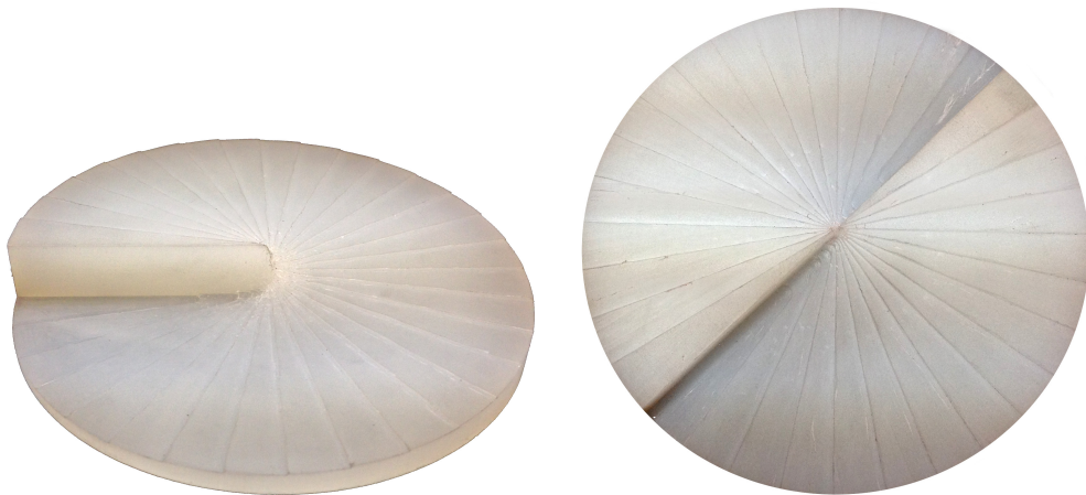
(b) Split Configuration \Delta l = \pm 2 SPP. (c) Standard Configuration \Delta l = \pm 2 SPP.
