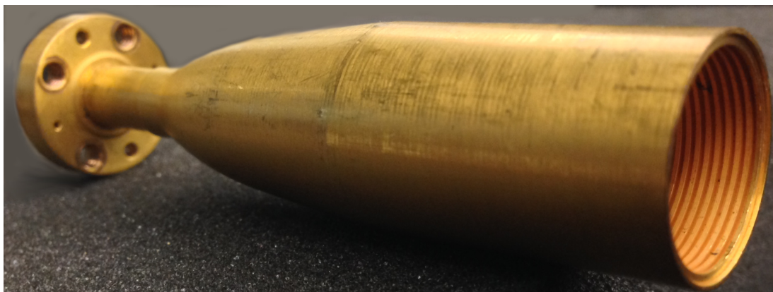
Figure 6.4: Corrugated feed antenna used to generate divergent Gaussian beams.
