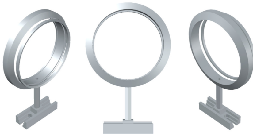
Figure 7.8: CAD renderings of the SPP mount designed for these experiments. A slotted base is used to position the mount on an optical bench or three-axis positioning stage. The mount surface and support are angled to minimise reflections and reduce standing waves. A SPP is placed inside the mount and secured with a threaded backing ring.
