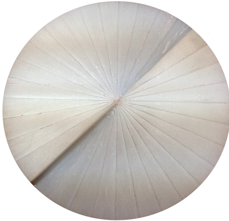
Figure 4.5: A split stepped polypropylene \Delta l = \pm 2 SPP.
