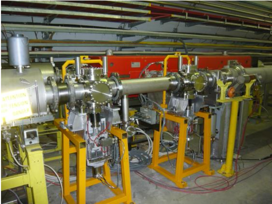
Figure 2.6: Installation of the SPS scrapers in the LSS1.
