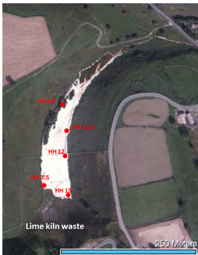
Figure 1 Aerial photography of Brook Bottom Spring at Harpur Hill in Buxton. Sampling points, and corresponding pH values at the time of sampling are also shown (Ordnance Survey data 2013; Grid reference at centre: SK 056 717).
