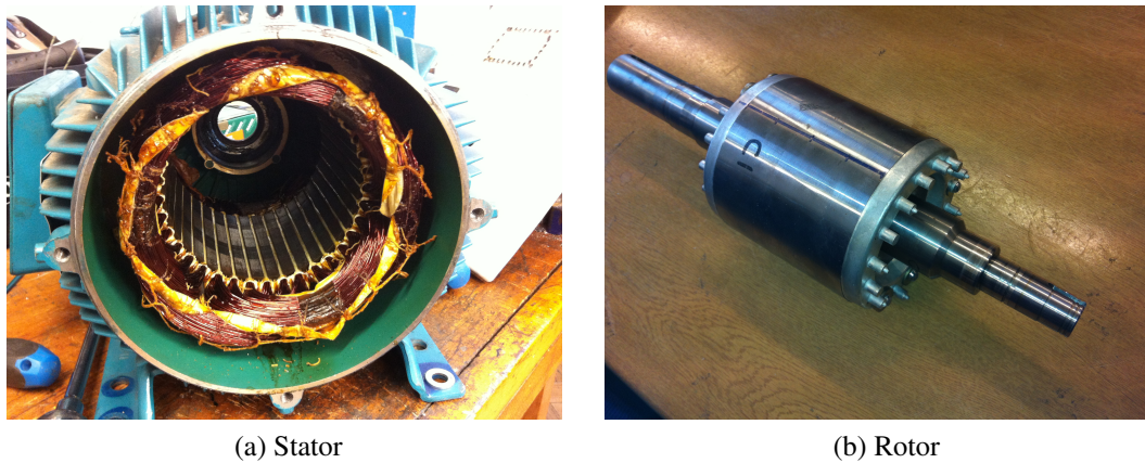
Figure 3.3: 5.5 kW industrial induction motor
