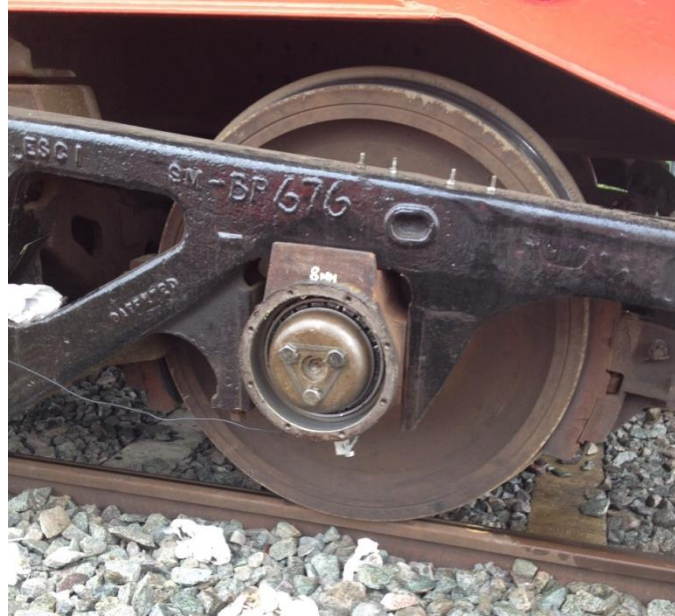
Figure 6-21: Photograph showing one of the faulty axle bearings with an artificially induced 8 mm deep roller defect.
