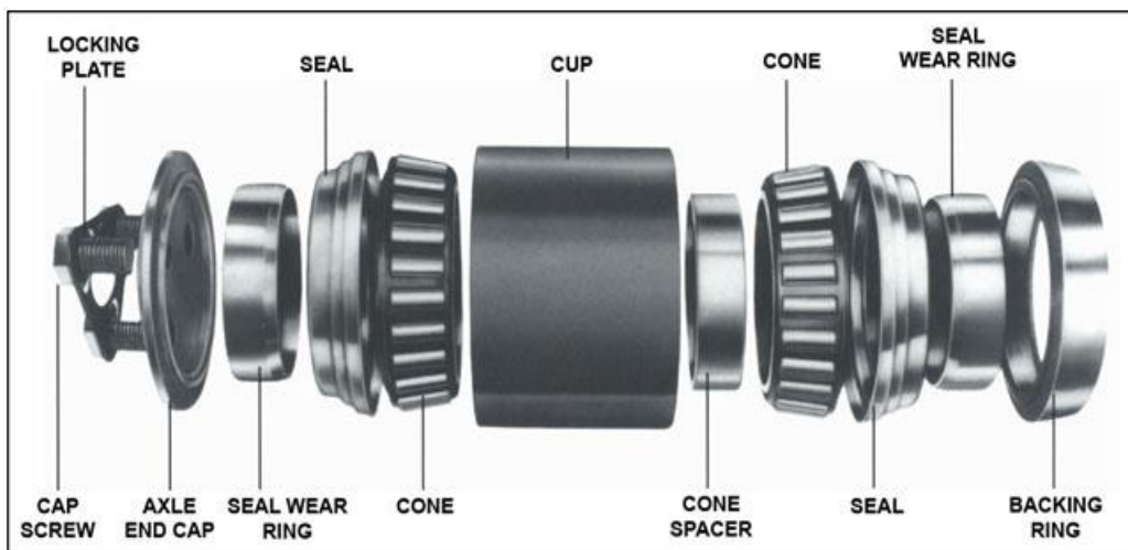
Figure 2-4: Schematic of a tapered roller bearing (courtesy of TIMKEN AP).
