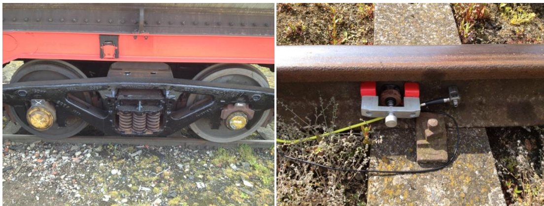
Figure 6-22: Photographs showing aspects of the experimental configuration employed for the Long Marston trials. On the left one of the bogies with one faulty axle bearing containing a roller defect (right wheelset) and a healthy axle bearing (left wheelset). The photograph on the right shows an acoustic emission and vibration sensor pair mounted on the rail web.
