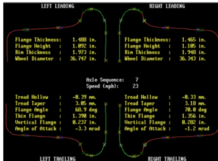
Figure 4-2: Typical output of wheel profile detector (Bladon et al., 2004).
