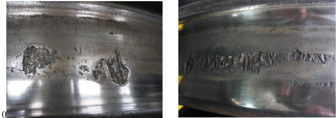
Figure 2-2: Shelling on the wheels of the test vehicle due to braking.
