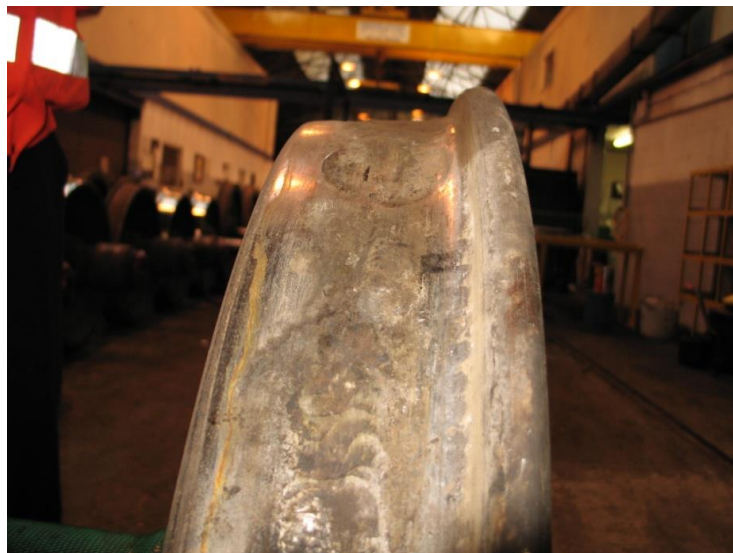
Figure 2-3: Photograph showing wheel flats on the tread of a wheel.
