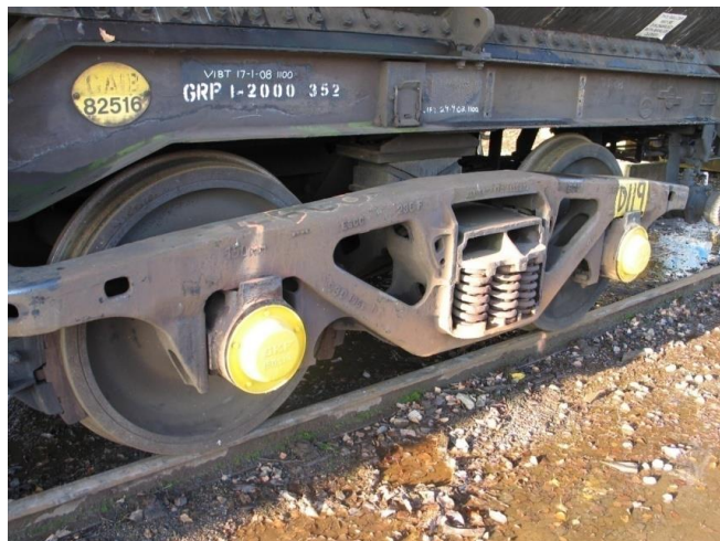
Figure 2-6: Photograph showing a typical freight bogie.
