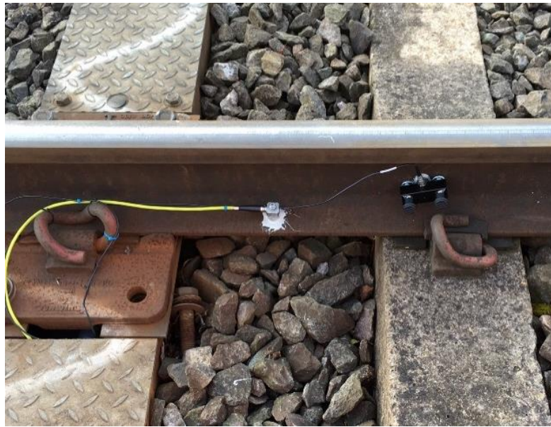
Figure 6-25: Acoustic emission and vibration sensor pair mounted on the rail at the Cropredy site.
