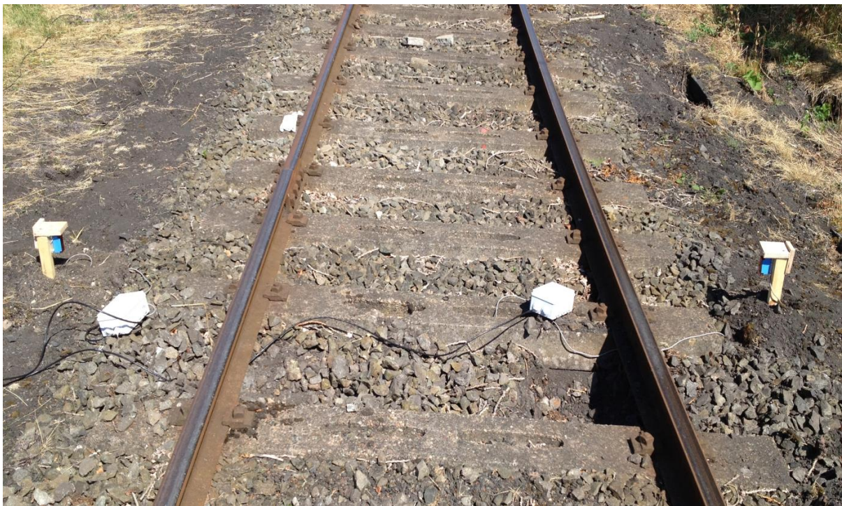
Figure 6-13: One of the IR transmitter-receiver pairs comprising the optical triggering system after installation at the Long Marston test track.
