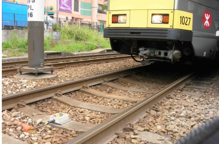
Figure 4-8: Example of AVI system (Photograph courtesy of Citycom).
