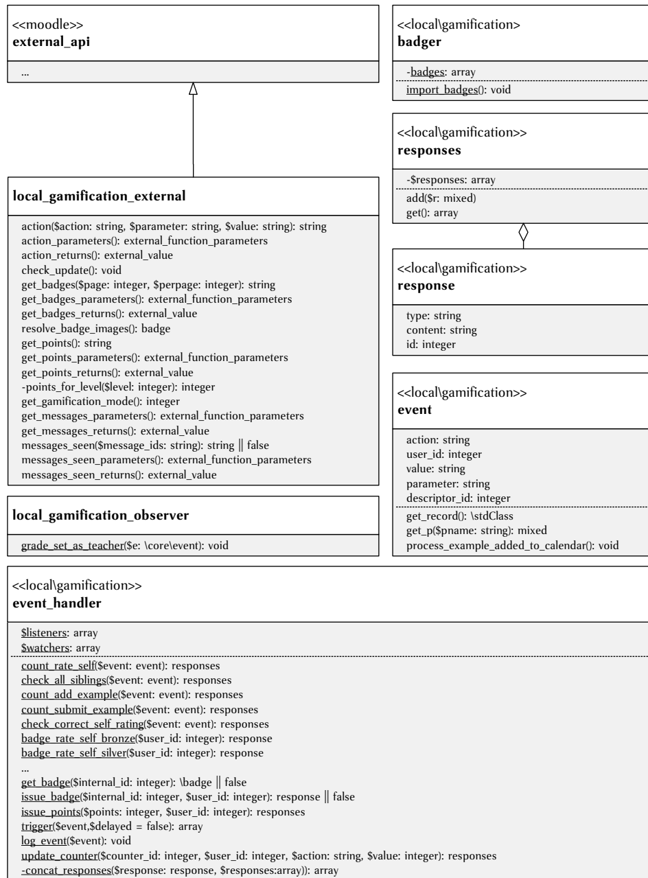
Figure 5.9: Class diagram of the Moodle plug-in. Includes some simplification for readability's sake. Own illustration.
