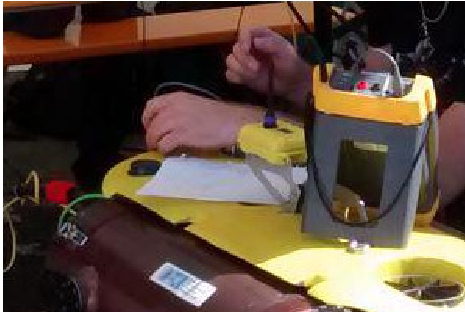
Figure 2.24: Dagon's WiFi access point, which can be used instead of copper cables, is housed in a waterproof box (yellow in the middle).
