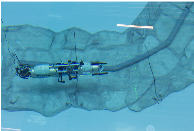
Fig. 7 Avalon is inspecting the pipeline in the maritime test hall at DFKI Bremen ( 23m x 19m x 8.0m ) (picture: Anemarie Hirth / DFKI GmbH)
