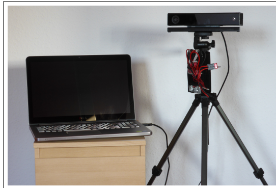
Figure 3.1: The acquisition setup used consisted of the Microsoft Kinect Camera v.2, tripod, and Dell Inspiron Notebook.
