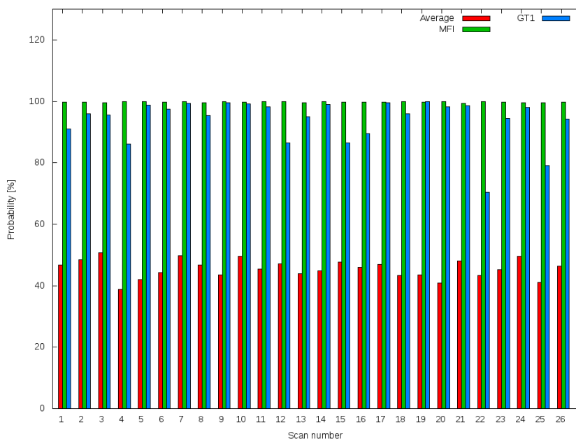
Figure A.3: Probability to find the object table at different positions (grid resolutions of 0.01 meters).
