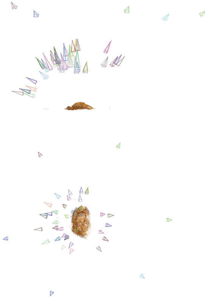
Fig. 6 Screenshot of a visualization of the camera positions used to image a single folio side, indicating the range of movement required around the folio to gain enough coverage of the surface to build a robust model
