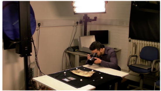
Fig. 4 Kazim Pal undertaking the digitization process, which required much movement around each folio. You can also see here a set of small ceramic balls placed around the folio which we originally had planned to use for calibration: these were not required as our work progressed but they remain in the capture shots. Video 1 (which is available in the online version of this paper) shows a time-lapse of a typical capture sequence, indicating the range of angles required to gain a complete coverage of each folio side, and indicating that the digitization process was non-contact
