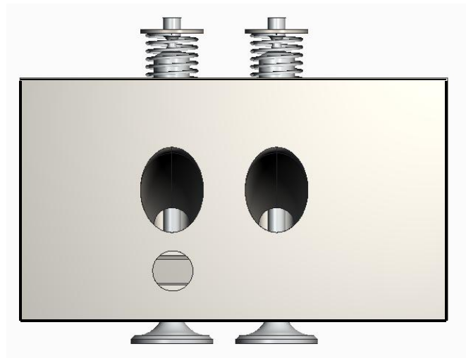
Figure 6.2: Side view of newly designed cylinder head model
