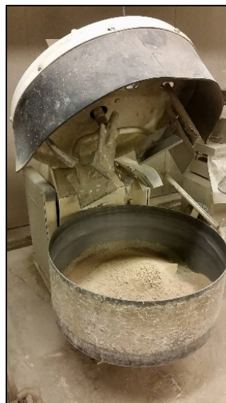
Figure 9 Pemat mixer in concrete lab, Aalto University.
