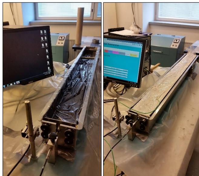
Figure 11 Picture of Early Age Autogenous Deformation Test with the Schleibinger Bending-Drain.
