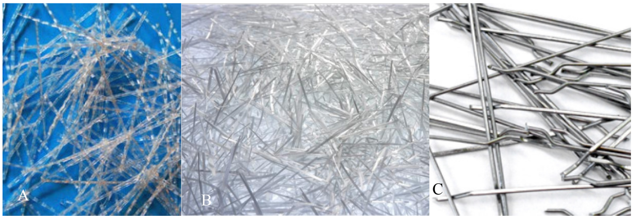
Figure 6 A) Plastic (polypropylene) fibres. (BASF, 2016) B) Glass fibres. (Owens Corning, 2015) C) Steel fibres. (ArcelorMittal, 2010).
