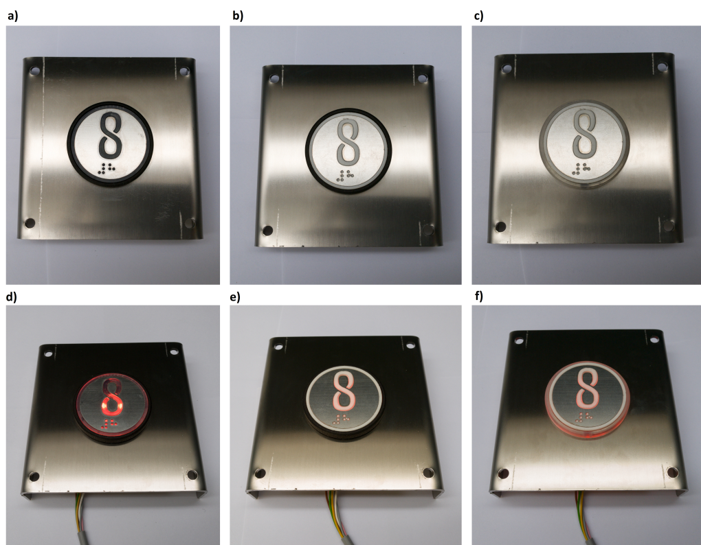
Figure 6.1: The final elevator button assembly in different material combinations. a) a PA2200 base colored black with a clear faceplate, b) a PA2200 base colored black with an untreated white PA2200 faceplate, c) a clear base with an untreated white PA2200 faceplate, d) , e) , f) forementioned assemblies illuminated in the same order.
