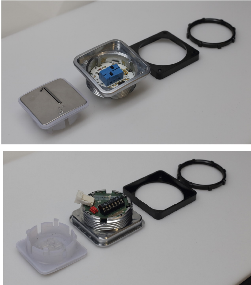
Figure 4.1: A traditionally manufactured elevator button disassembled. Components from left to right: a faceplate and spring package glued on the backside, an externally threaded base with the circuit board glued, an offset collar, and the fastening nut.
