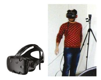
**Figure 5: The study using virtual reality:** a) The HTC Vive VR headset used for the experiment. b) A person wearing the headset and participating in the experiment.
