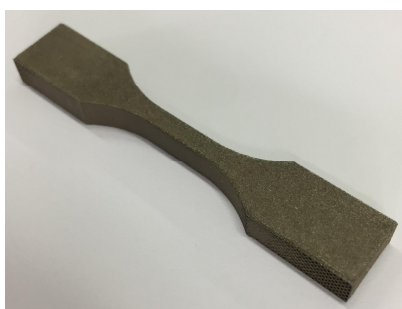
Figure 66. A specimen of additively manufactured Stainless Steel 316L with dimensions of 60mm x 10mm x 5mm.
