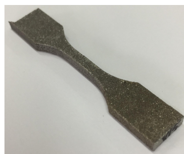
Figure 67. A specimen of additively manufactured Titanium Ti64 with dimensions of 60mm x 10mm x 3mm.
