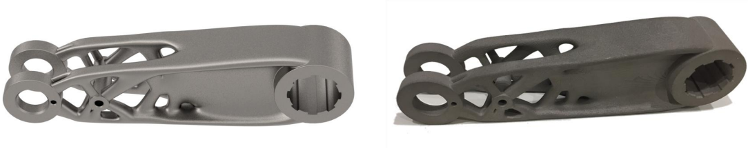
Figure 65. A Rendered Image of CAD model (Left) and metallic prototype (Right) of the final optimized model of Upper Shank.
