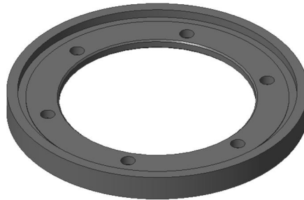
Figure 15. A CAD model of Cutting Blade containing a bounding box of 183mm x 183mm x 16mm.
