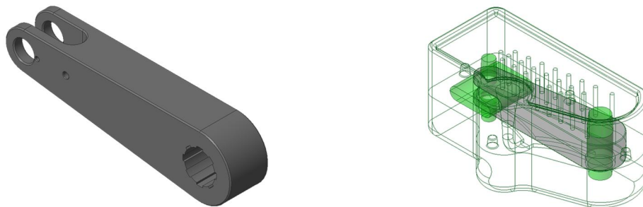
Figure 13. A CAD model of Upper Shank (Left) and its sand mould (Right) containing a bounding box of 455mm x 125mm x 77mm and 566.4mm x 316.1mm x 263.5mm, respectively.
