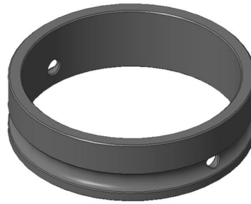
Figure 23. A CAD model of Stopper Flange Assembly containing a bounding box of 90mm x 90mm x 25mm.
