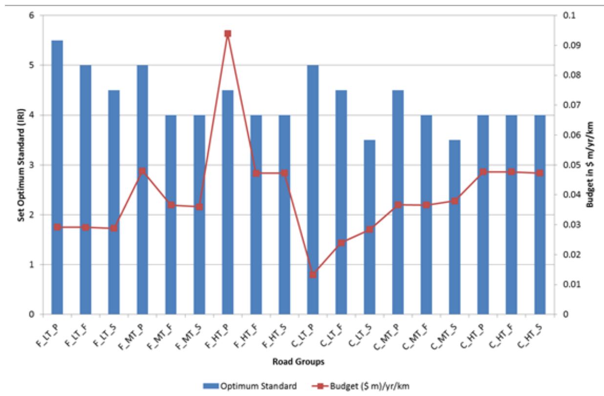
Figure 7.1: Derived optimum maintenance standards and required budget for the flexible and composite roads
