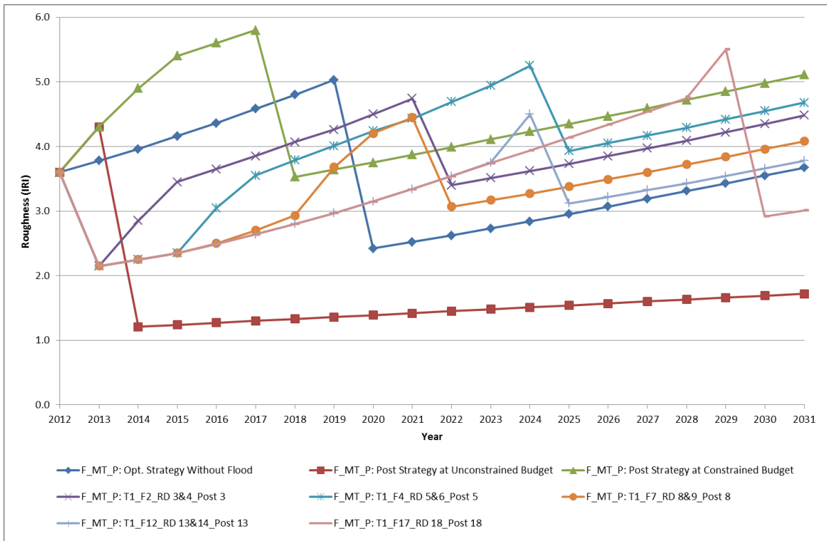
Figure 9.11: Pavement life-cycle performances at the optimum, pre- and post-flood strategies for the F_MT_P road group
