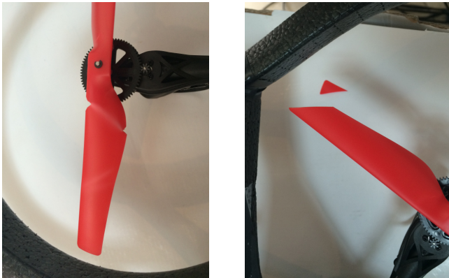
(a) Cut and bended propeller. (b) Cut propeller.
