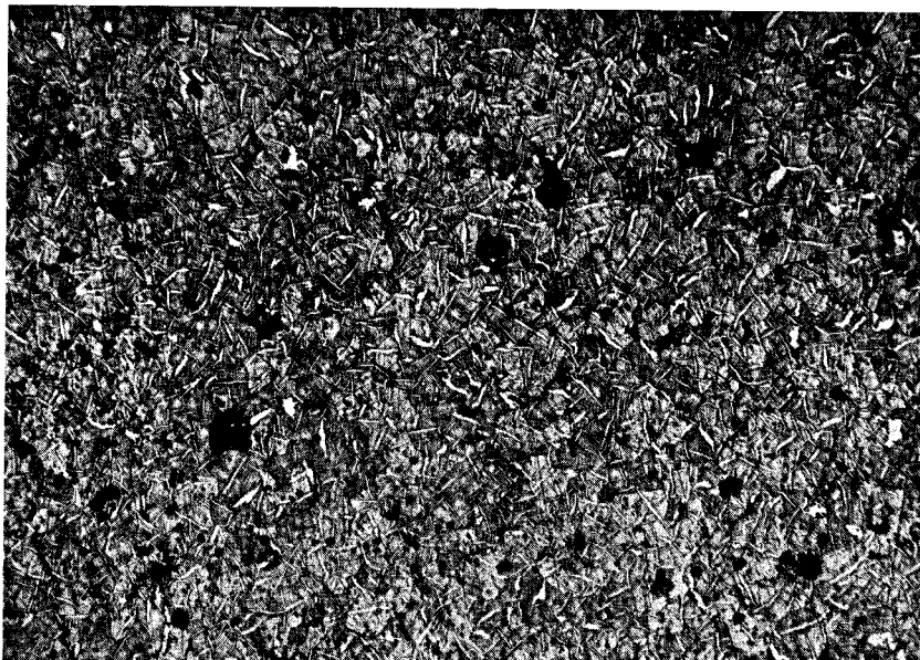
Fig. M 8c O/Pu = 1,69 200 \times Spec. 20, quenched from 500 \text{ }^\circ\text{C} . The structure now is clearly two phase.
