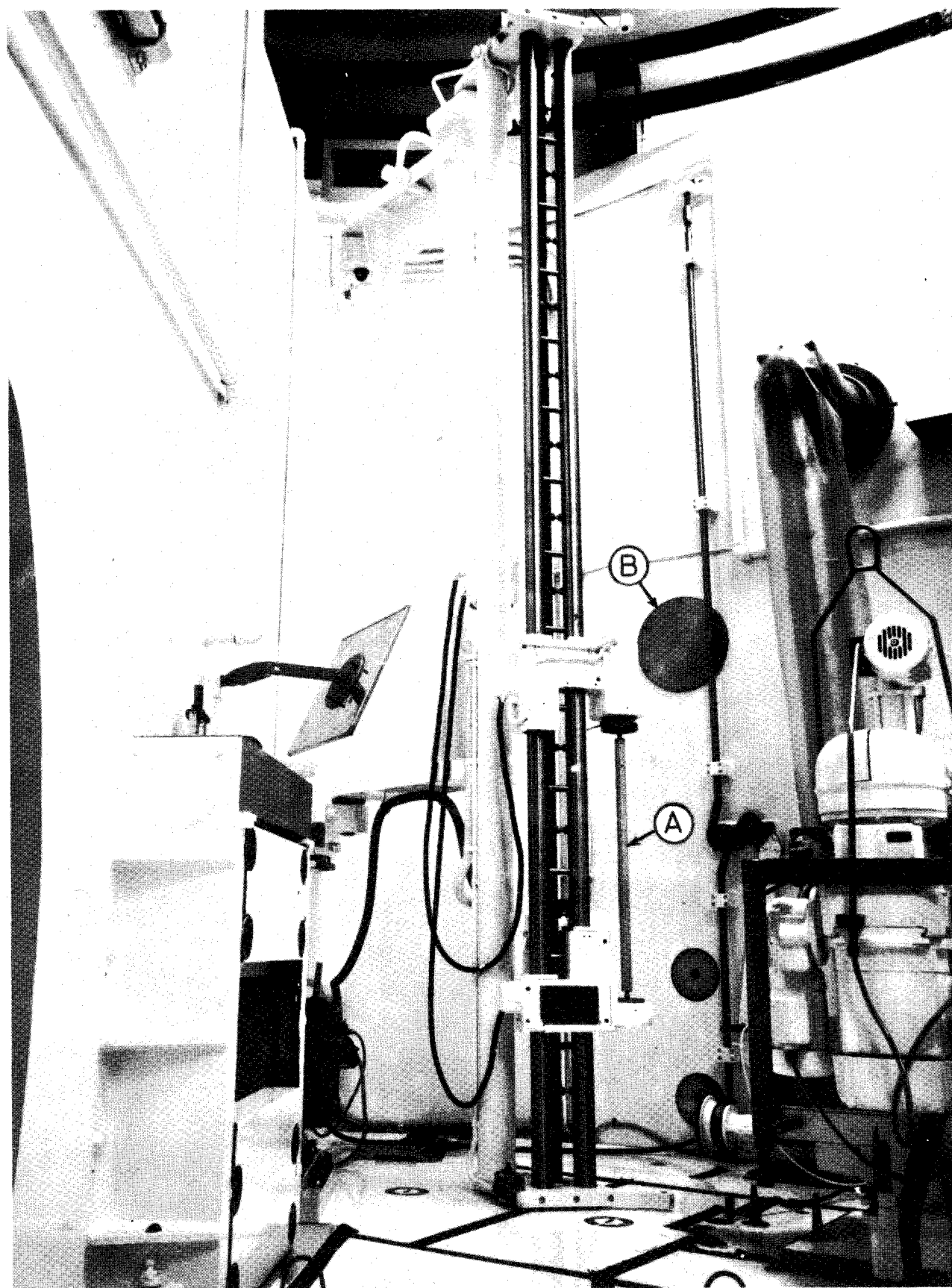
Fig. 17 - Gamma scanning equipment. A. Fuel rod B. Collimator
