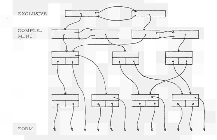
One more facility was provided for the handling of syntactic homographs (total or only partial during analysis). Elements (at the form level) and relations are linked to the upper level not directly, but by means of a nodal point ("link-list") which administrates the alternative use of each of them.
