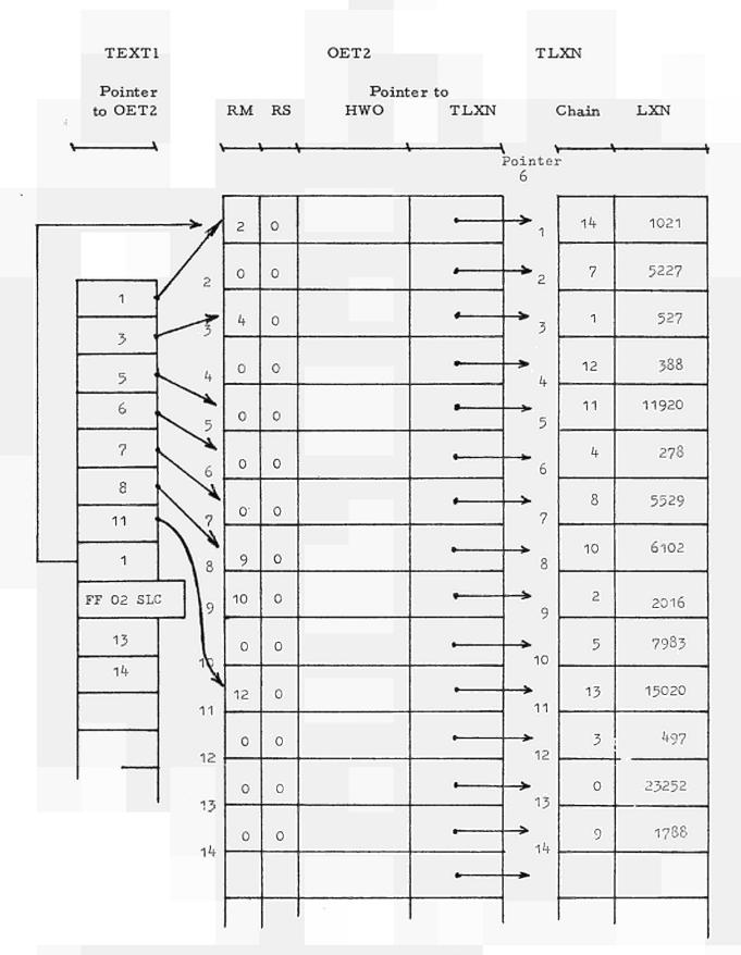
Fig. 12 - Data Structure before Dictionary Loading
