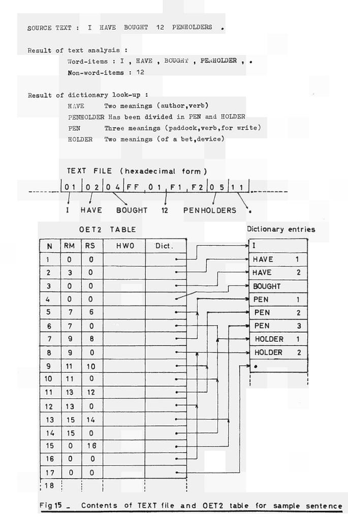
the application), and each one of these units is organized in core storage as a four-levels tree structure (item - match - segment - form), called TEXT IMAGE, the nodes of which are linked to all the informations obtained from the precedent phases. Part of the functions of SLC-II programming language was specially designed to handle this tree structure and to access the different data.
