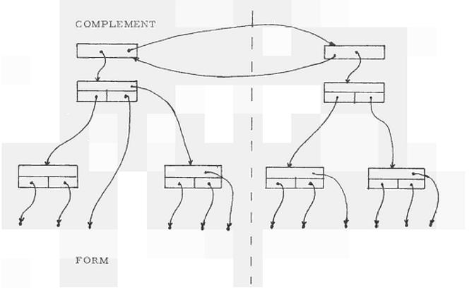
All alternative solutions, which, in principle, cannot be put into relation with each other, are grouped together at the highest level of the syntactic text representation ("exclusive level").
