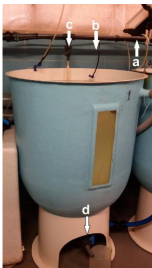
Figure 6 Blue tank of 300L. The letters correspond: a) automatic feeder; b) aeration tube; c) water renewal tube; and d) purge site.
