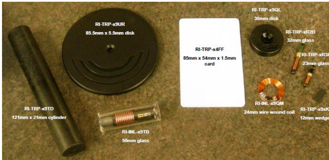
Fig. 2.2 – Photograph of different types of RFID tags, developed by Texas Instruments™ [41].
