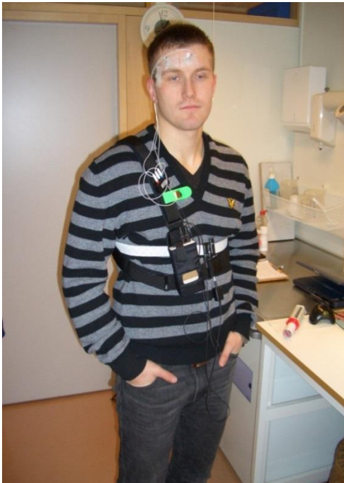
Figure 5: (Left) Volunteer equipped with EMG electrodes for recording of blinking frequency, an inductive flexible chest belt for recording of breathing frequency and a data logger (black box). (Right) Recordings of the blinking and breathing frequencies
