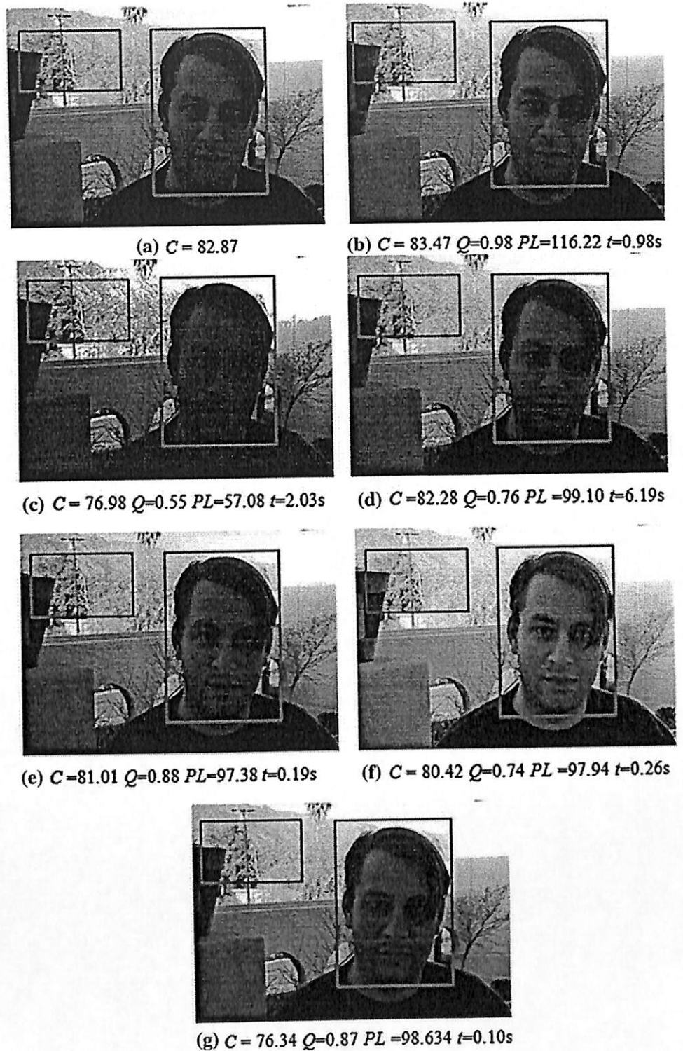
Fig. 5 Comparison of the enhancement results a Original Man 2 image, b the proposed AFIM method, c FQM [48], d DCT [56], e BPDFHE [46], f TM [39], g GC ( \gamma=0.8 ) [24]
