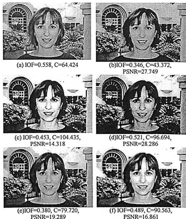
Figure 2: (a) original image (Woman), enhanced image with (b) proposed method (c) NINT (d) quantitative measure (e) fuzzy rule-based (f) fuzzy local enhancement
