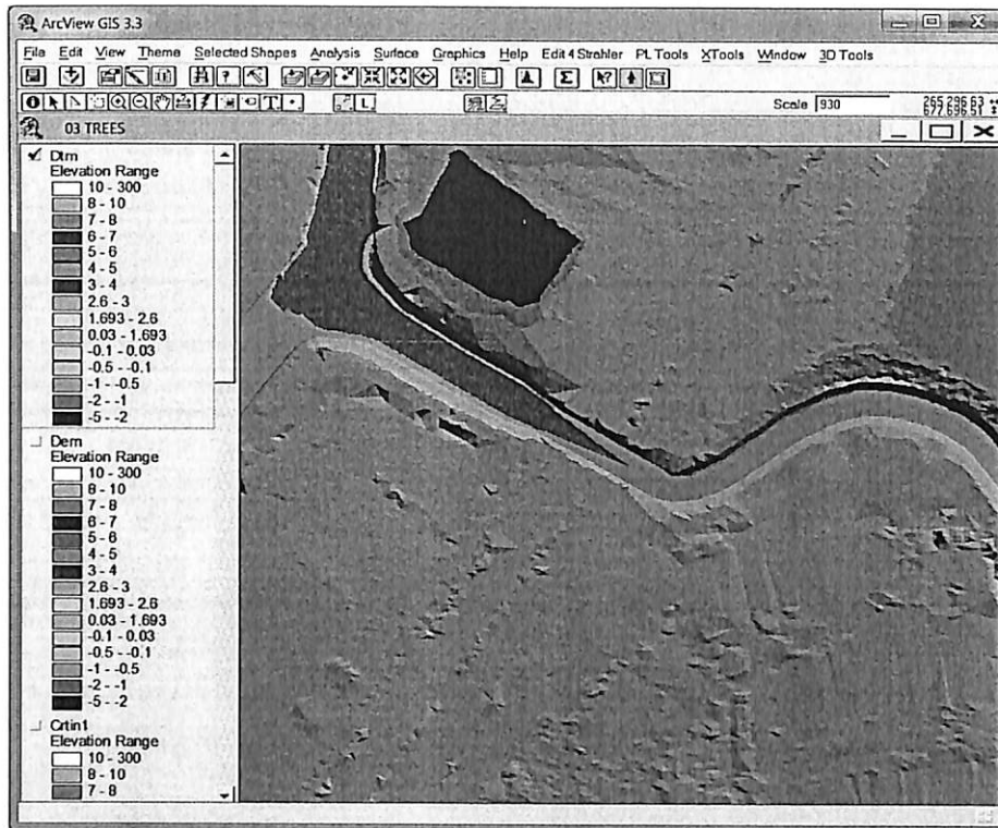
Figure 3.32: DTM was developed from DEM with trees and “high objects” removed.
