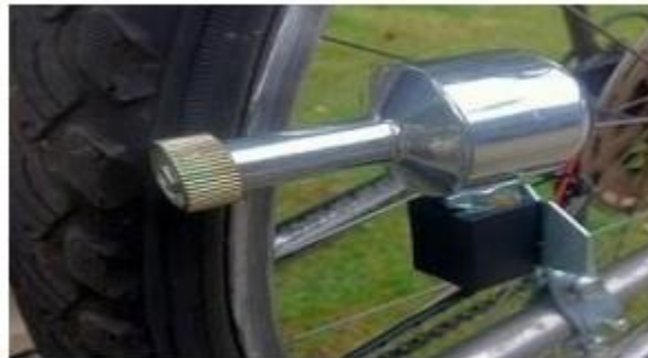
Figure 2.5: Bottle Dynamo mounted aside a bicycle wheel (Waliullah et al. , 2014)
