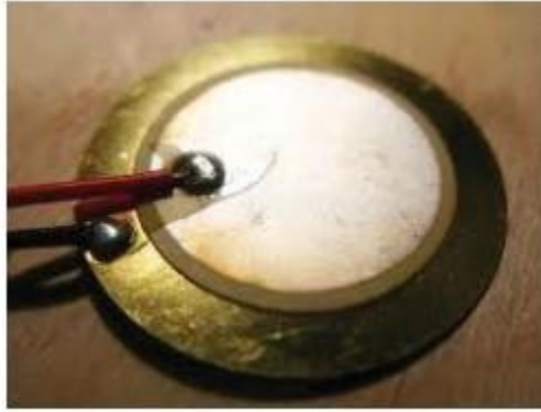
Figure 2.8: Piezoelectric disc (Pandey et al. , 2014)
