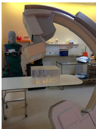
Figure 3. Set-up of anthropomorphic phantom in angiography room.
