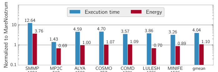
Fig. 13: Mont-Blanc vs MareNostrum: Performance and Energy comparison for a fixed number of MPI ranks.
