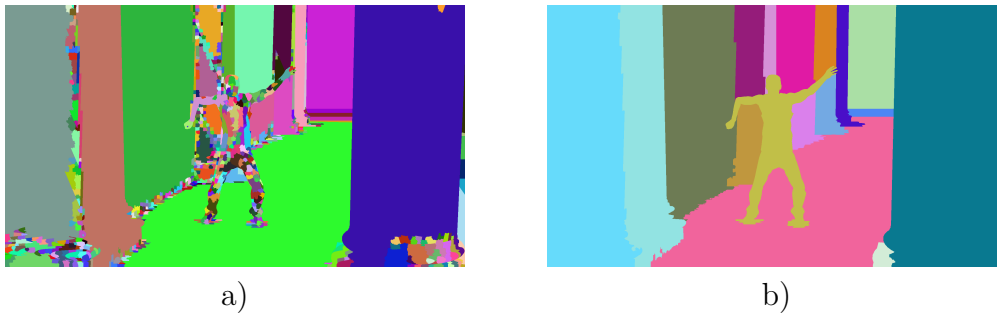
Figure 3.6: Depth Map Partition process. a) Result of applying the region growing algorithm. b) Final coding partition after the 3d_bpt algorithm.
