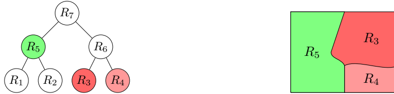
Figure 4.1: Lagrangian optimization over hierarchies. The bottom-up analysis follows the merging sequence from Figure 3.1 activating the nodes with minimum lagrangian. The algorithm finds the best partition (regions 3, 4 and 5) and the best coding strategy.
