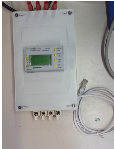
Figure 22: The analyser mounted in the protective case
