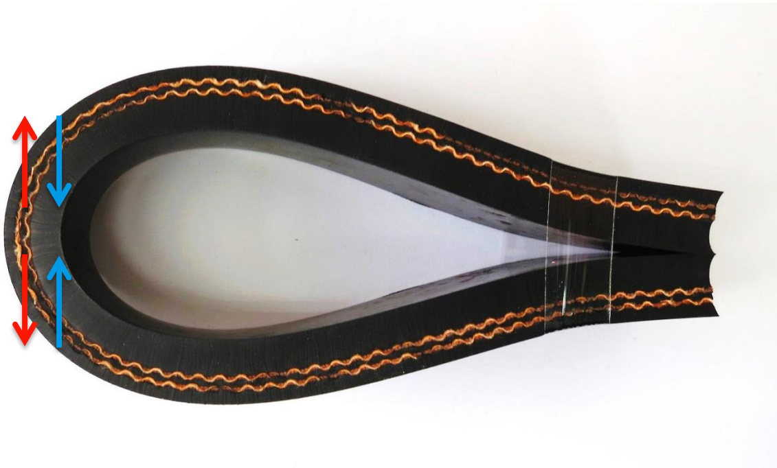
Figure 4: Bending characteristics of membranes for inflatable dams
