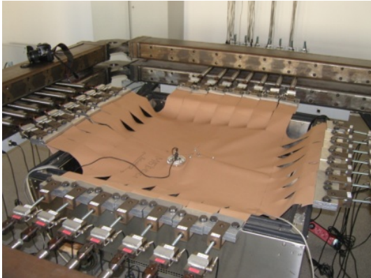
Figure 4: Biaxial-testing, prepared sample
