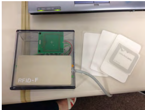
Figure 7 IC tag card and IC tag reader (see online version for colours)
