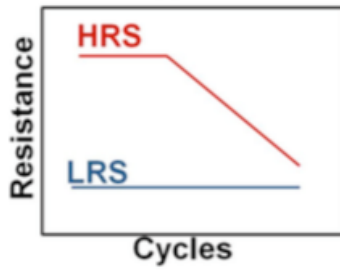
Fig. 5 Degradation model showing the depletion of O_2 induced HRS reduction [5].
