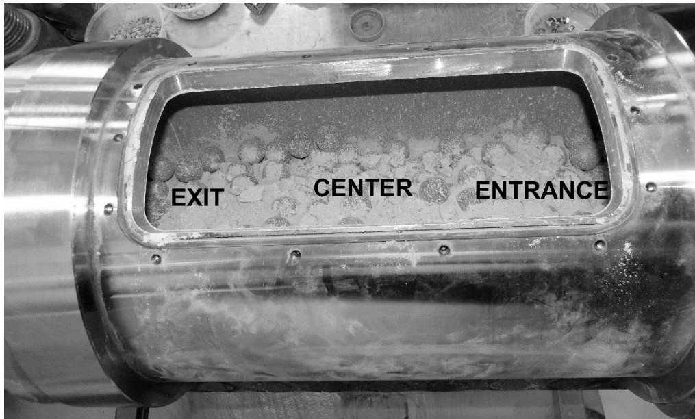
Figure 1. Interior of the mill during an experiment. Coarse particles are fine compacted aggregates dropped from the window.
