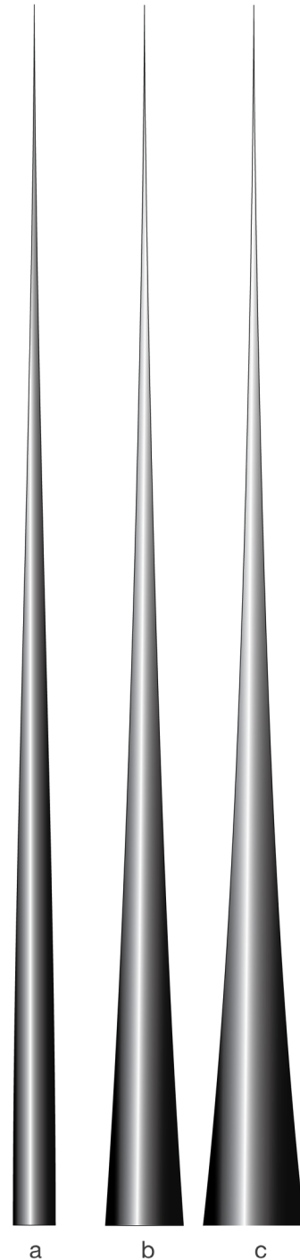
Figure 1: Tallest column profiles (a) Linear elastic (b) & (c) Non-linear elastic, stress limited
