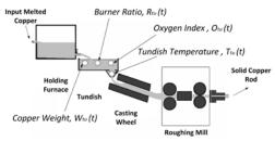
Fig. 5. Diagram of the copper rod manufacturing process [22].
