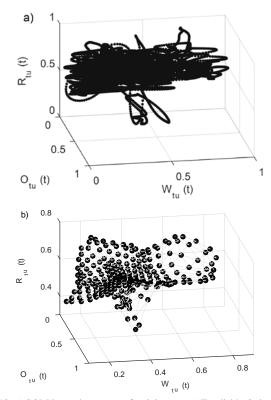
Fig. 10. a) SOM input data space of training set: x) Tundish's Oxigen value in ppm, y) Tundish burner's ratio in % and z) Copper weight in the tundish in Kg. b) Neurons of the SOM grid after the training procedure.
