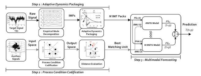
Fig. 1. Block diagram of the design procedure of the proposed multimodal modelling method. The procedure is divided in three steps: (i) Adaptive dynamics packaging, (ii) Process condition codification, and (iii) Multimodal forecasting.
