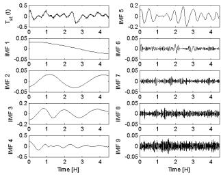
Fig. 7. Intrinsic mode functions extracted from the tundish's temperature of the training set during a time window processing.
