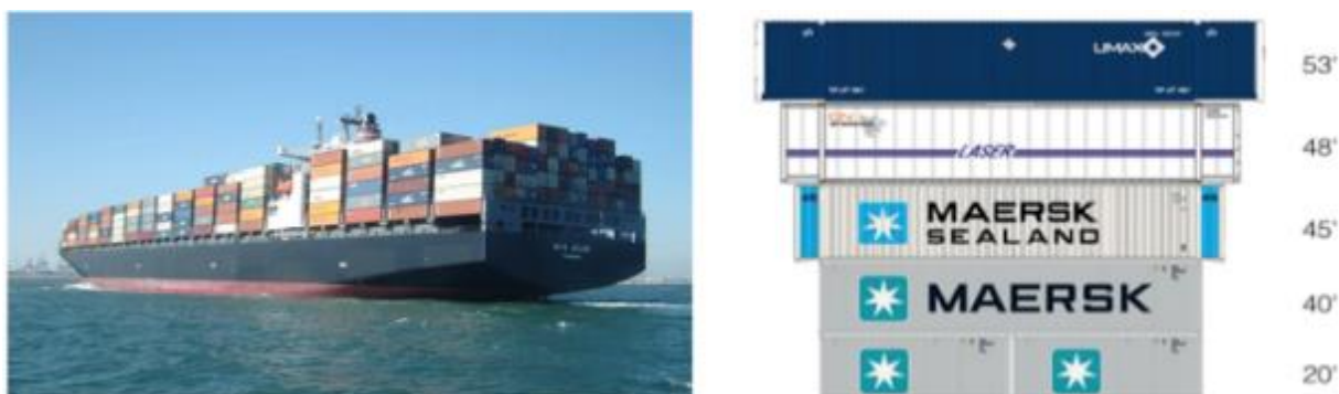
Figure 2: Sea Containers on a cargo ship (left) [2] and various container sizes (right) [3]
