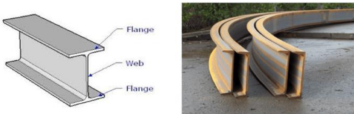
Figure 51: I-profile and bended C-profile which will be used for the rounded part [25]
