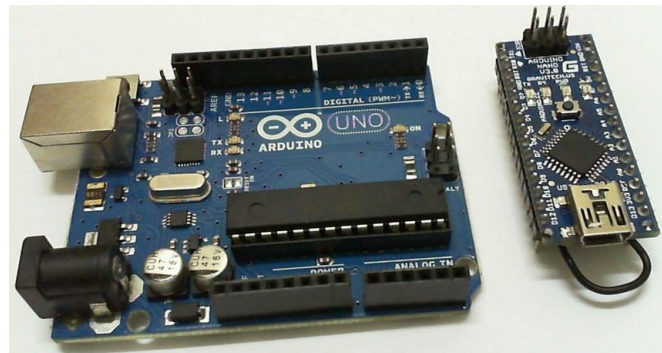
Figure 49: Comparison between Arduino Uno and the new Nano
