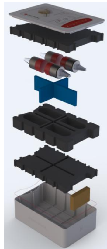
Figure 18: Explosion View of Smart Packaging
