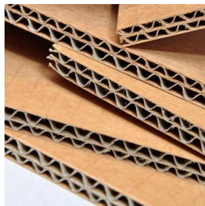
Figure 29: Double Walled Board
