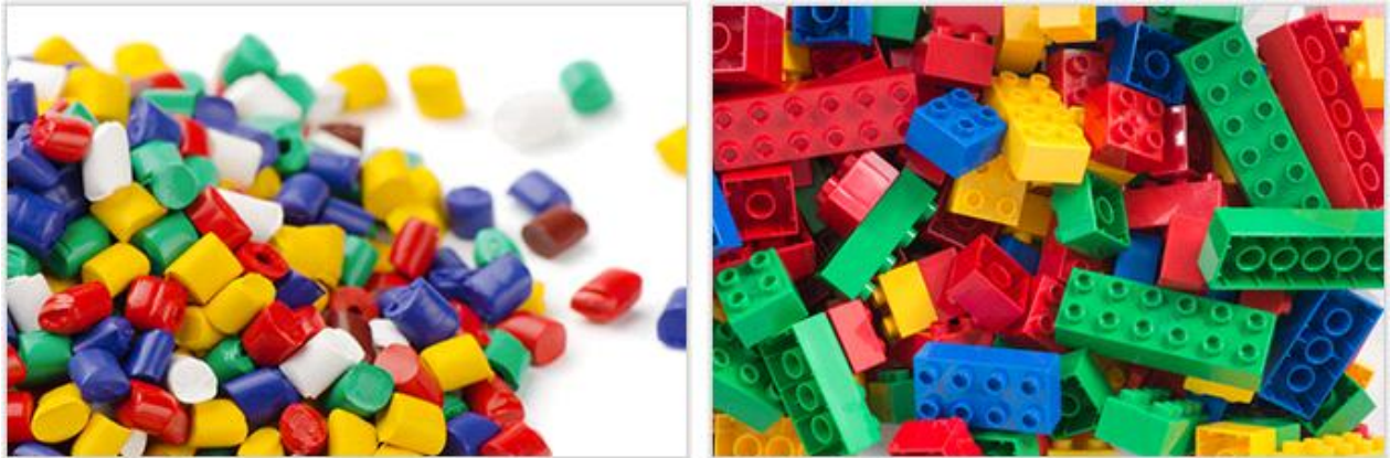
Figure 32: ABS Pellets and ABS Lego Toys
